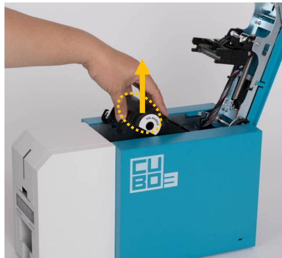
Figure 11 Take out the ribbon cartridge
