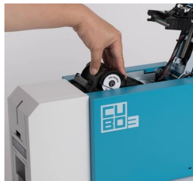
Figure 16 Installing the ribbon cartridge
