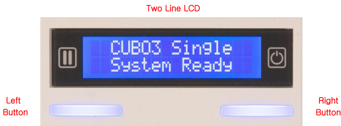
Figure 7 CUBO3 Display and Buttons
