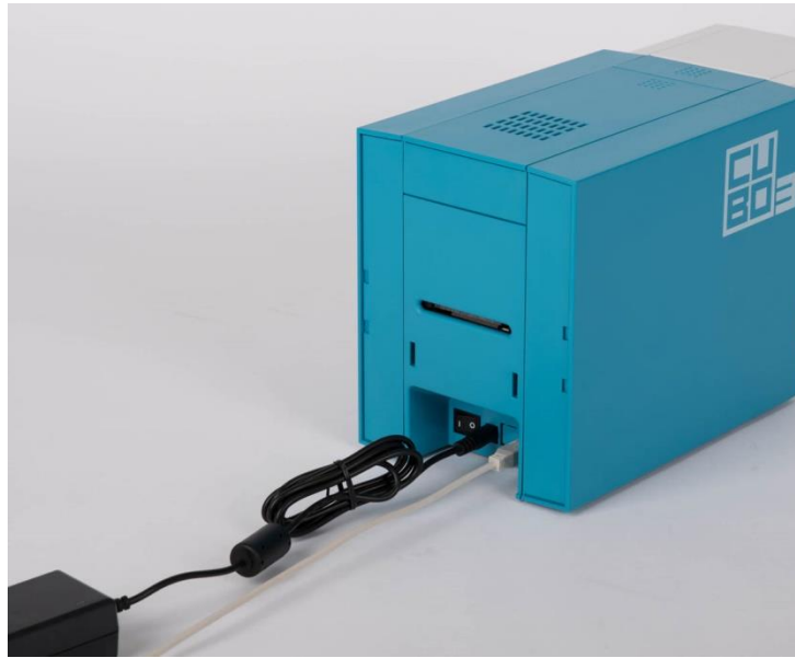
Figure 8 CUBO3 single Connection of power and USB cable
